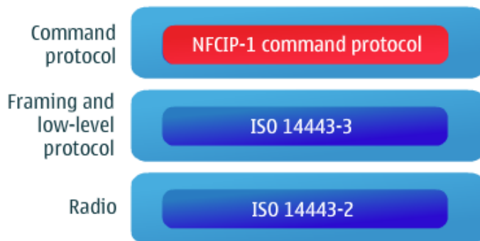
Figure 6: ISO 14443 protocol stack
