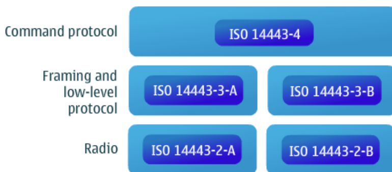
Figure 5: ISO 14443 protocol stack
