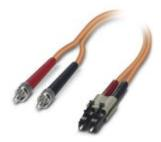
Assembled FO cable, zip cord cable, multi-mode fiberglass 62.5/125 µm, OM1, connector: FSMA/LC duplex, degree of protection: IP20, for installation in cable ducts or control cabinets
