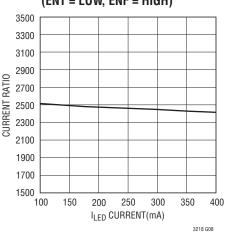
Flash I<sub>LED</sub>/I<sub>SET</sub> Current Ratio vs I<sub>LED</sub> Current (ENT = ENF = HIGH)
