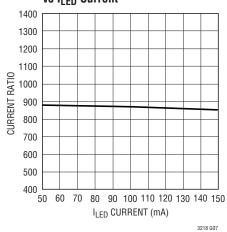
Flash I<sub>LED</sub>/I<sub>SET</sub> Current Ratio vs I<sub>LED</sub> Current (ENT = LOW, ENF = HIGH)
