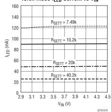
Flash Mode I<sub>LED</sub> Current vs V<sub>IN</sub> (ENT = ENF = HIGH)
