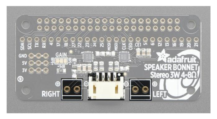
This is the fun part, you get stereo output - one left and one right channel. You can use the JST 4-pin plug in the center if you're going to just plug in one of our enclosed speaker kits:
