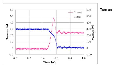
Fig. 14 IGBT Turn-on. Typical turn-on waveform at Tc =  $100^{\circ}$ C,  $V_{CC}$  = 300 V, Ic = 25 A
