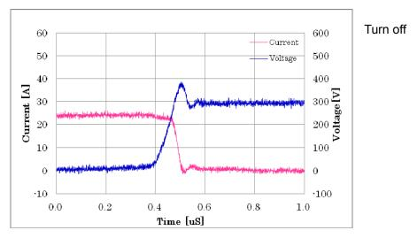
Fig. 15 IGBT Turn-off. Typical turn-off waveform Tc =  $100^{\circ}$ C,  $V_{CC}$  = 300 V, Ic = 25 A
