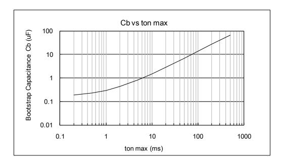
Fig.16 Ton-max vs CB characteristic
