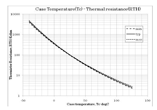
Fig.11 Variation of thermistor resistance with temperature
