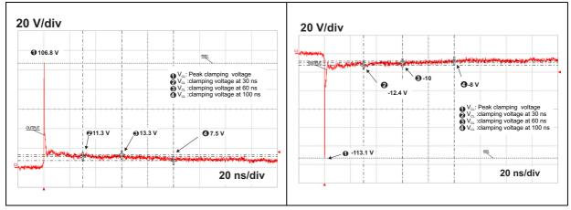
Figure 17. TLP measurements
