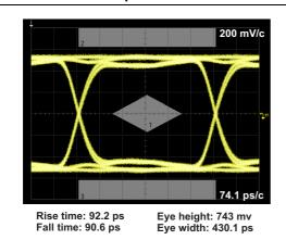
Figure 11. Eye diagram SD4.2, 3.12 Gbps Thru PCB
