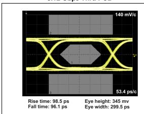
Figure 13. Eye diagram USB2.0, 480 Mbps Thru PCB
