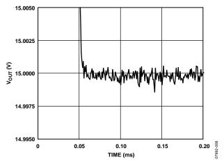
Figure 8. Output Settling Time (High to Low)
