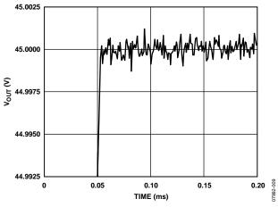
Figure 9. Output Settling Time (Low to High)
