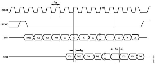
Figure 4. Read Timing Diagram
