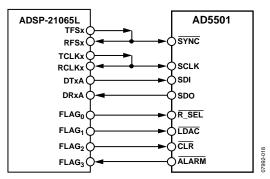
Figure 19. Interfacing to an ADSP-21065L DSP
