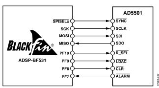
Figure 18. Interfacing to a Blackfin DSP
