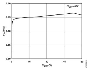
Figure 11. I<sub>DD</sub> vs. V<sub>OUT</sub>
