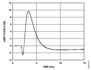
Figure 13. Digital-to-Analog Positive Glitch Impulse
