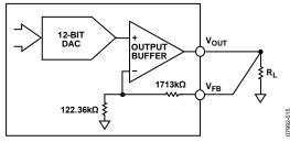
Figure 15.  $V_{FB}$  and  $V_{OUT}$  Configuration
