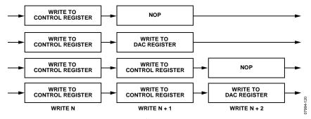
Figure 17. Control Register Write Sequences
