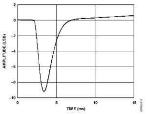
Figure 12. Digital-to-Analog Negative Glitch Impulse
