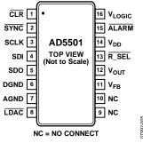
Figure 5. Pin Configuration
