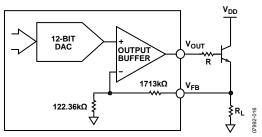
Figure 16. Pass Transistor Configuration
