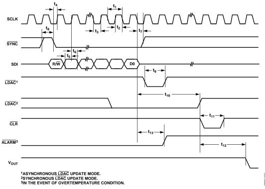
Figure 3. Write Timing Diagram
