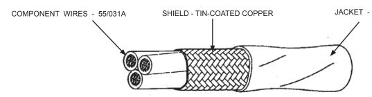
JACKET - LOW OUTGASSING, RADIATION-CROSSLINKED, MODIFIED ETFE
