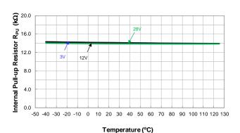
Internal Output Pull-up Resistor vs Temperature
