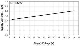
Supply Current vs Supply Voltage
