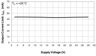
Output Current Limit vs Supply Voltage
