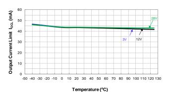
Output Current Limit vs Temperature
