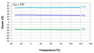
Switch Points Bop and Brp vs Temperature
