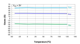
Switch Points Bop and Brp vs Temperature
