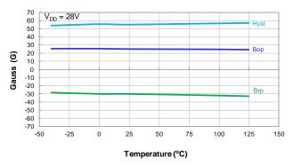
Switch Points Bop and Brp vs Temperature
