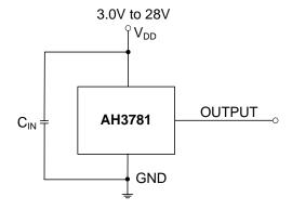
Note: 4. C<sub>IN</sub> is for power stabilization and to strengthen the noise immunity, the recommended capacitance is 10nF ~ 100nF. R<sub>L</sub> is the pull-up resistor.
