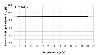
Internal Output Pull-up Resistor vs Supply Voltage
