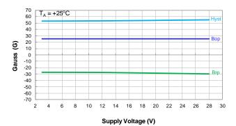
Switch Points Bop and Brp vs Supply Voltage
