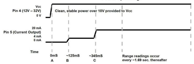
A = Power is applied and is stable at the proper voltage
