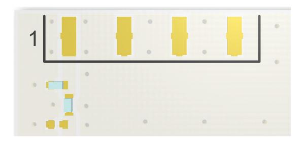
Below the footprint is shown again but without the solder mask. Pin 1 feed must be connected to GND as shown here.
